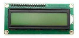
An LCD display is one of the most frequently connected devices to а microcontroller. Among the most common types are 16x2 and 20x2 LCD displays, which represent 16 characters per line across 2 lines and 20 characters per line across 2 lines, respectively. LCD, or Liquid Crystal Display, is a flat-panel display technology that utilizes liquid crystals to produce images. These displays are widely used in various electronic devices, including televisions, computer monitors, smartphones, and more.
